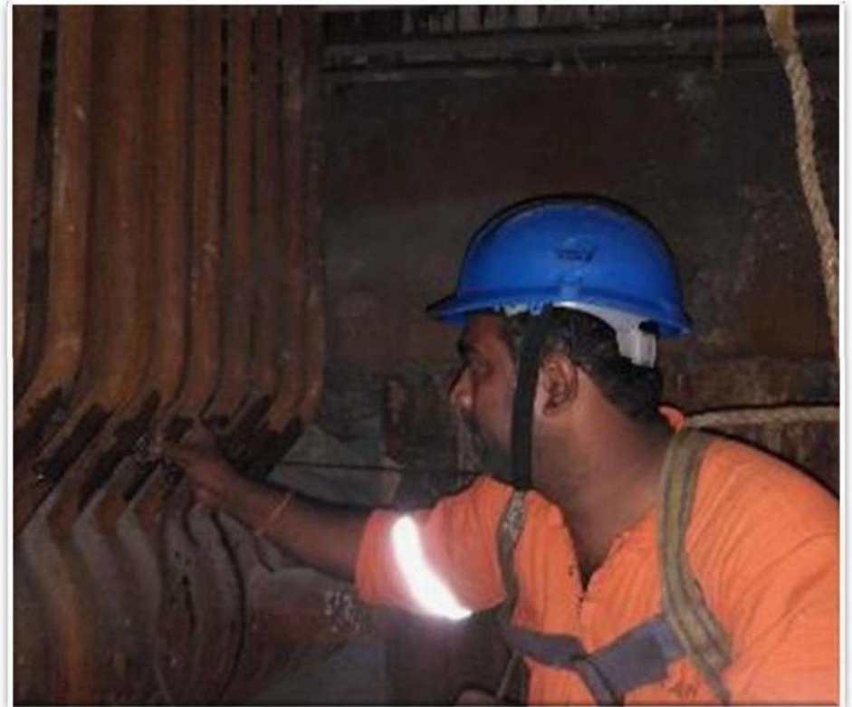
PAUT Inspection of Boiler Tubes for GE(Power) at MPL ,Jharkhand
