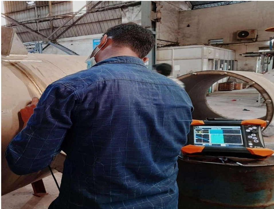
PAUT Demo for IGCAR at TEAM, Chennai Using Gekko on Stainless steel welds
