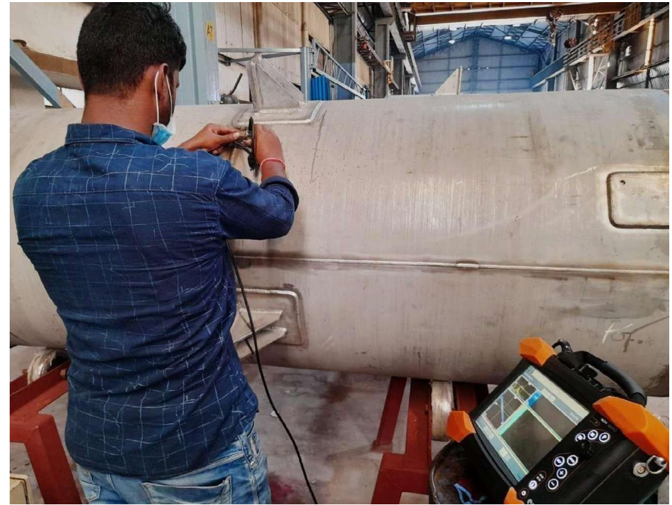
PAUT Demo for IGCAR at TEAM, Chennai Using Gekko on Stainless steel welds
