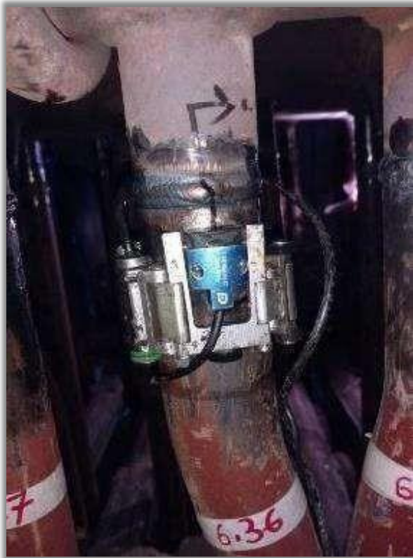
PAUT of Power Plant Piping Using Cobra Scanner at Sonichar, NIGER
