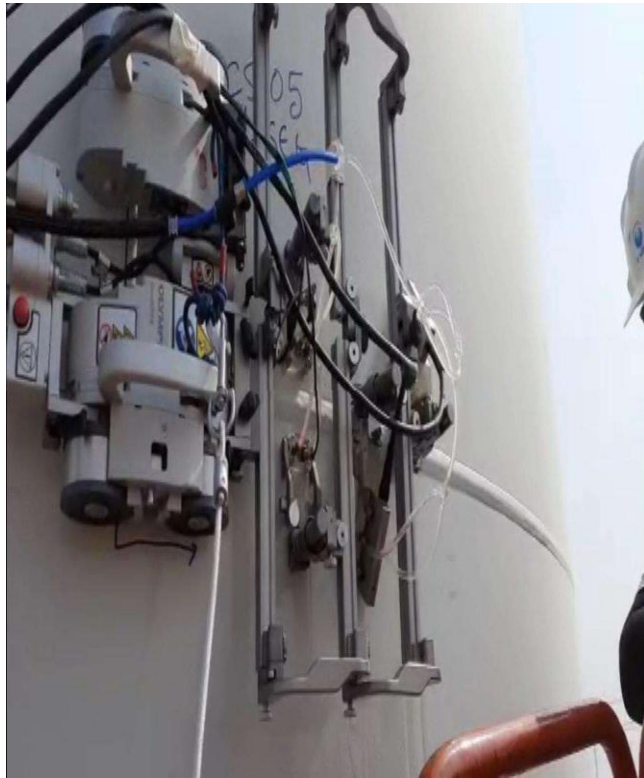
Inservice Inspection of windmill Tower Using SteerRover for SGRE in Bijapur, India
