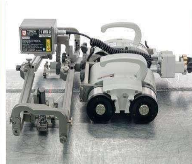
In-service Inspection of windmill tower weld using ToFD & PAUT with fully automatic scanner For Siemens Gamesa Renewable Energy (SGRE)
