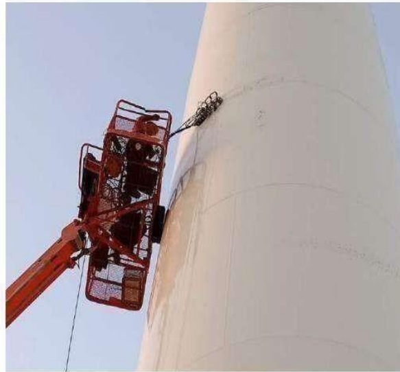
In-service Inspection of windmill tower weld using ToFD & PAUT with fully automatic scanner For Siemens Gamesa Renewable Energy (SGRE)
