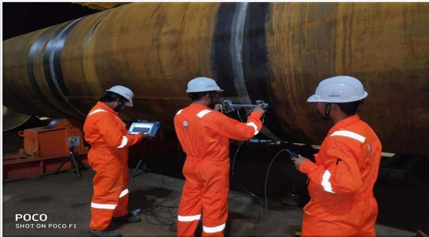
PAUT & TOFD Inspection of Structure joints at L&T MFF, Hazira
