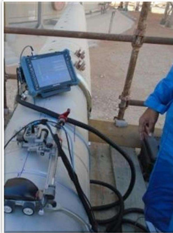
Hydroform Corrosion Mapping - Velosi Oman
