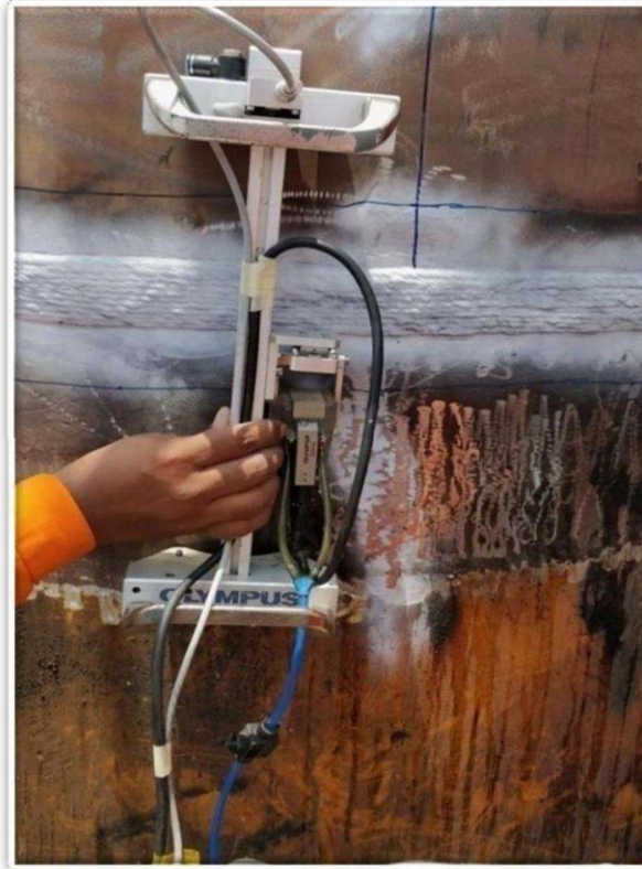
PAUT Inspection at ONGC Offshore Platform
