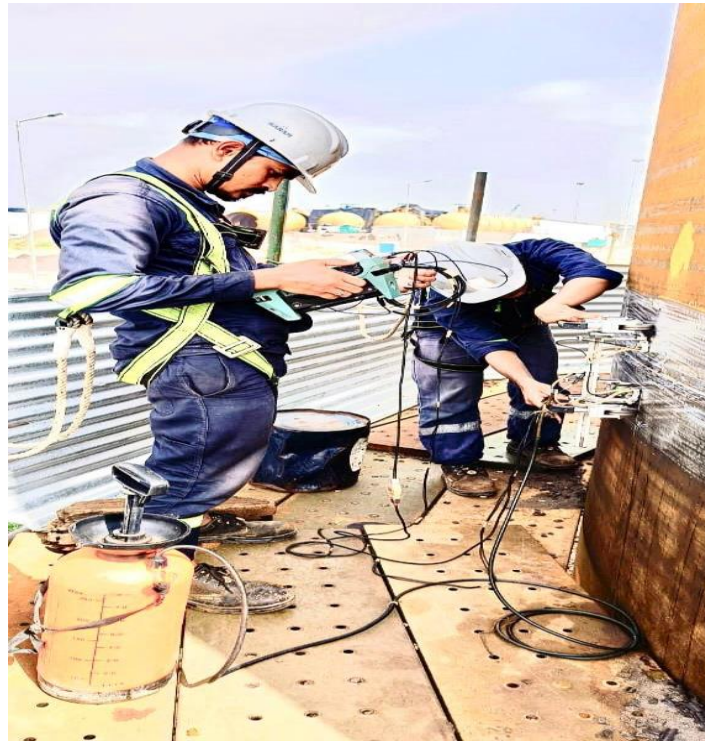
PAUT/ToFD Inspection of Mounted Bullets at Vijay Tanks & Vessels, HRRL, Rajasthan, India
